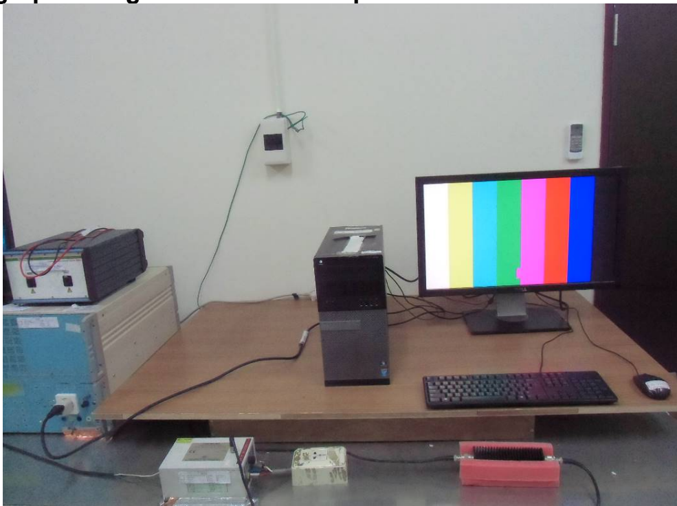
Photograph –Surge & EFT Test Setup
