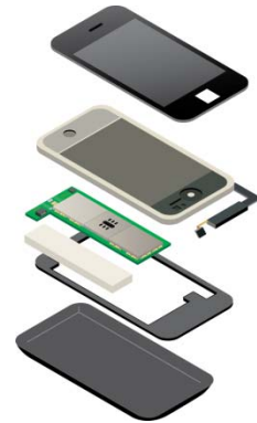
FG reinforcement between PCB and enclosure
