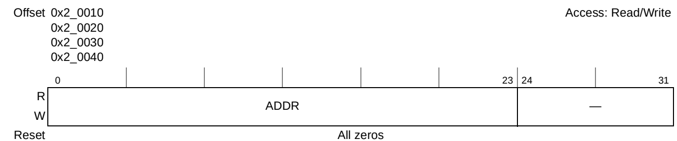
Figure 6-9. Cache External Write Address Registers (L2CEWAR n )
