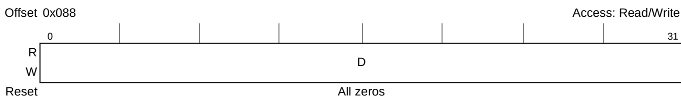
Figure 12-9. UPM Data Register in UPM Mode (MDR)
