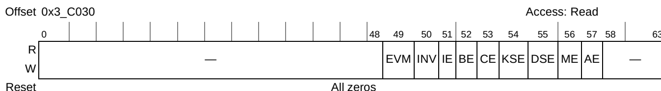
Figure 20-97. PKEU Interrupt Status Register
