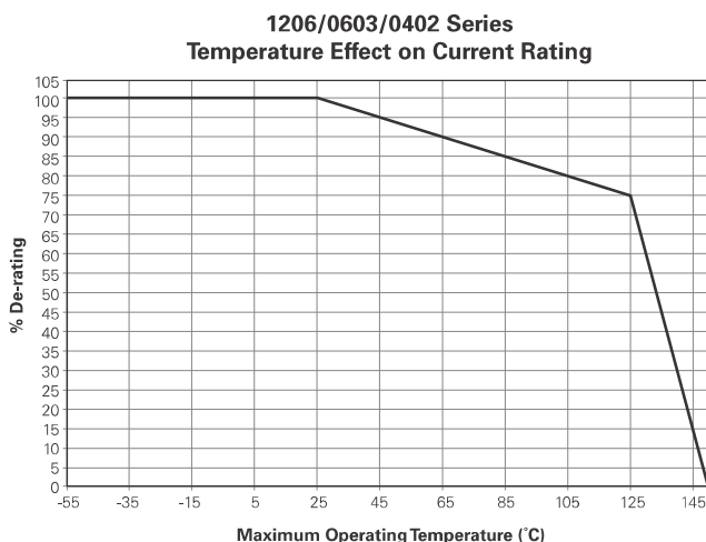
Figure F1 Thermal Derating Current for All Fuses
