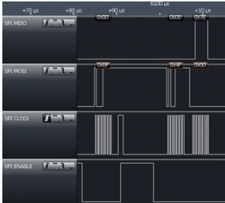
Figure 5-25. Reset FIFO and Read RSSI
